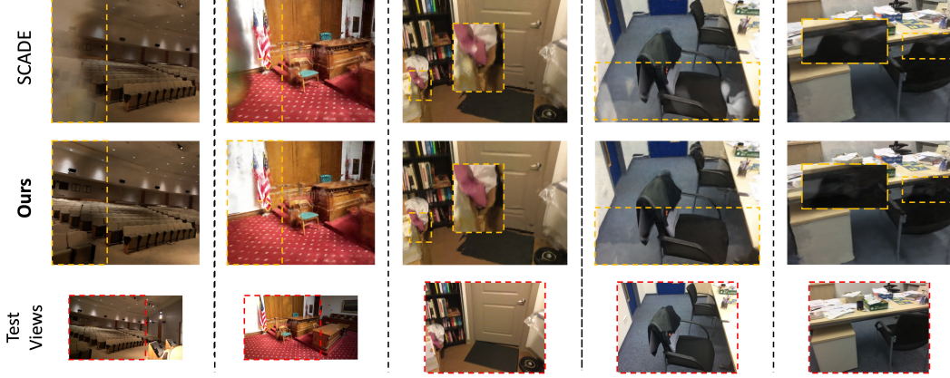
Figure 4: Visual Effect of \mathcal{L}_{\text{ProvNVS}} in Eq. 10. Compared to pre-trained SCADE model, our method can remove additional floaters in the scene (see the boxed region).
